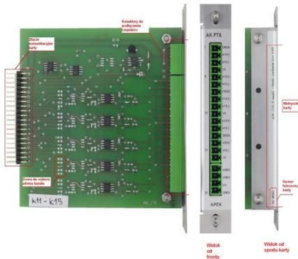
Measuring cards AK to AK32 system allow flexible system configuration. They can be change by the user. Cards are identified by type and serial number, each has described input numbers making easier configuration of APEK Assist program. The APEK Assist allows you, outside provided by manufacturer, a user's characteristics by modifying the tape of the card.
