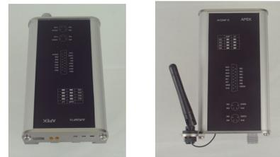
AV51 with the sensors socket of the type M12. On the right, the additionally external antenna.
