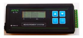
Aluminum body, with sides made from ABS, high quality membrane keyboard and window on backlit display.
